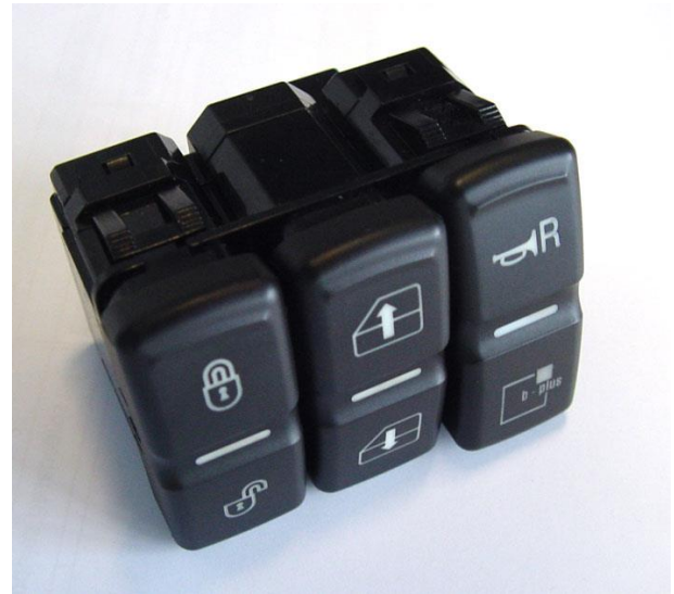
Illustration 1: Master Modul with SAE J1939 Interface, with customized Rockers and 3 way switch keys
