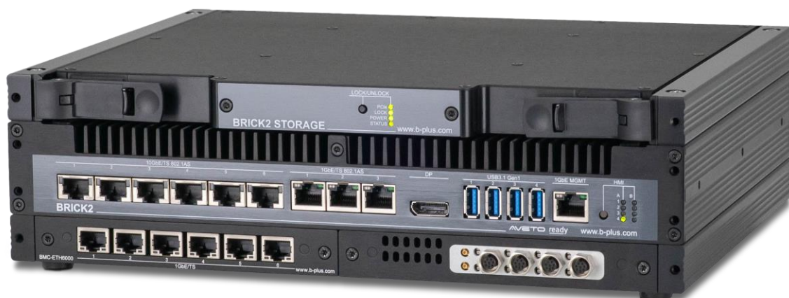
Figure 1.1: BRICK2 BMC with BMC-ETH 6000 and BMC-VB2
