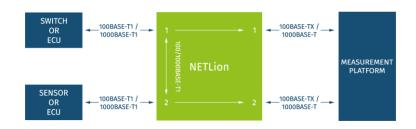
Decoupling of data of one 100/1000BASE-T1 line in both directions without influence of the communication
