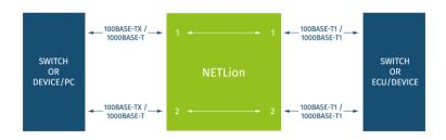
Conversion of two 100/1000BASE-T1 signals in standard 100BASE-TX/1000BASE-T Ethernet signals (bi-directional)
