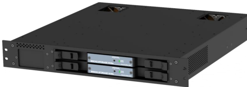
Add-on (bottom) for two BRICK2 STORAGE slots. The add-on is actively cooled and includes a PCIe 3.0 switch, µC based FAN control and power management. It supports cartridge Hot-Add/Hot-Remove and OS disk services for storage exchange during operation for NVMe based solutions.
