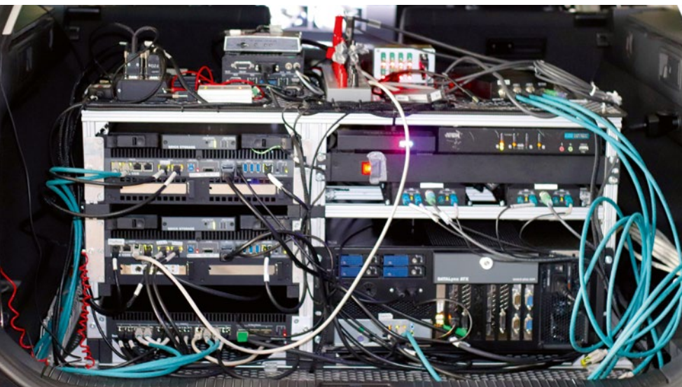
FIGURE 3 Possible b-plus measurement technology installation in a test vehicle (© b-plus)
