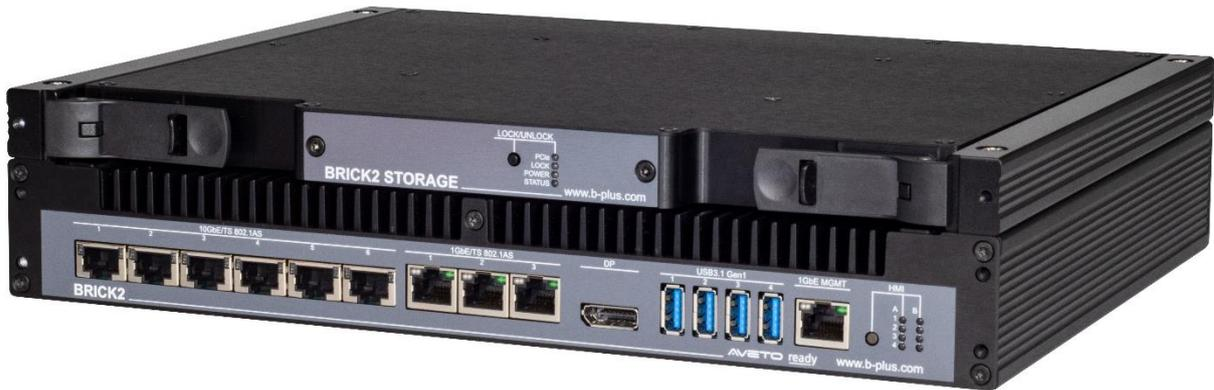
**BRICK2 is the next generation ADAS and AD measurement platform for the acquisition, processing and recording of high bandwidth data.**
