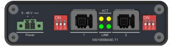
Figure 3: Interface for power, DIP switches for link configuration and 100/1000BASE-T1 interfaces
