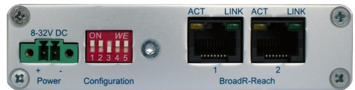
Illustration 4: Interfaces for power, DIP switches for configuration without SW-Tool and BroadR-Reach® interfaces
