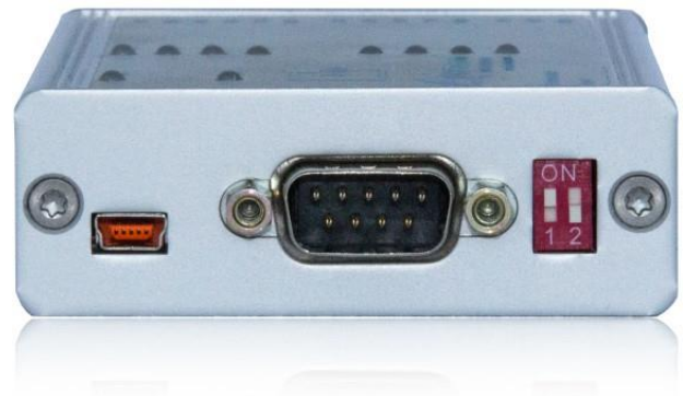
Illustration 4: USB Supply and SUBD-0 connector for termination switches
