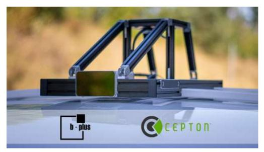
Image: Cepton's Vista-P60 lidar sensor is integrated into b-plus' AVETO tool box to enable the testing of sensor capabilities directly within the test vehicle MAX. @ b-plus technologies.
